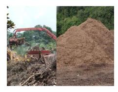
The above photo shows how Cisson has used a chipper and shredder to turn debris into mulch and compost but had been limited to grinding limbs and trunks that were 8 inches in diameter or smaller. They rented a tub grinder, which is capable of grinding even large tree trunks, to turn the debris into mulch at the nursery site, some 290 tons of yard waste had been accumulated at the nursery —the expense of having this disposed would have been \$11,000!
